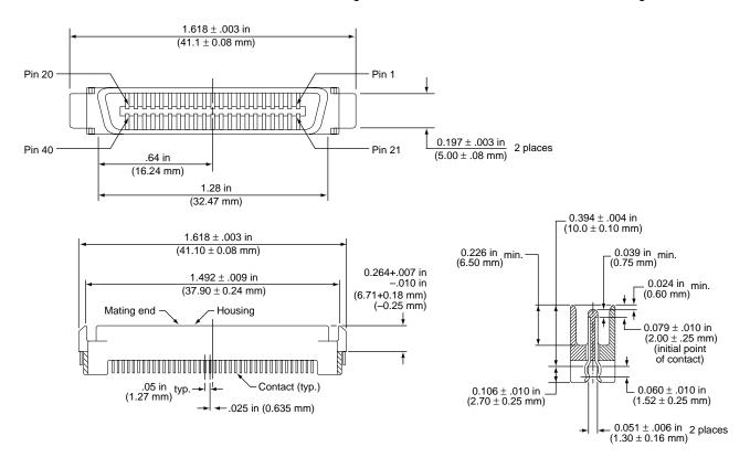
Figure 14. FC-AL SCA device connector dimensions
