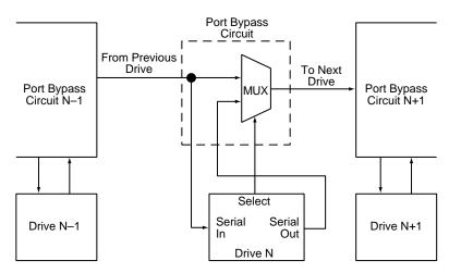
Figure 13. Port bypass circuit physical interconnect
