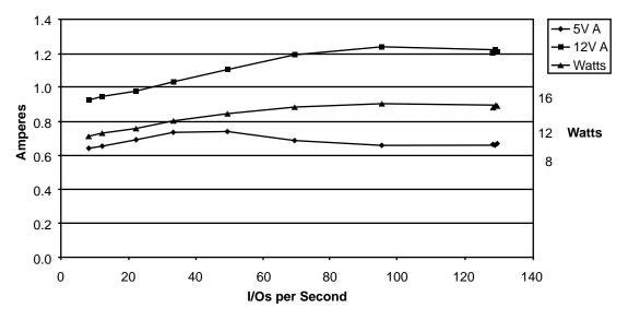
Figure 5. DC current and power vs. input/output operations per second
