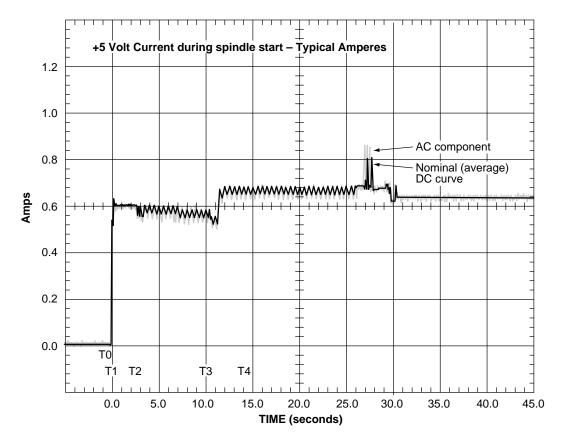
Figure 4. Typical Barracuda 36FC drive +5V current profile
