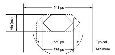
Figure 18. Receive eye diagram
