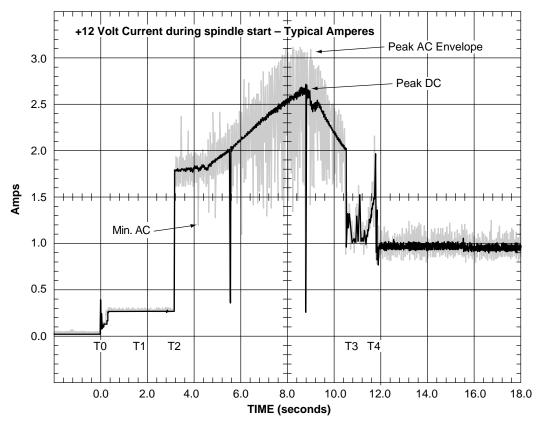
Figure 3. Typical Barracuda 36FC drive +12V current profile
