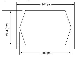
Figure 17. Transmit eye diagram
