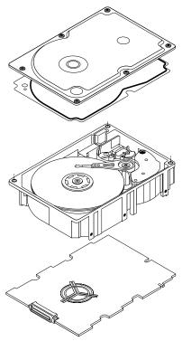
Figure 2. Barracuda 36FC disc drive
