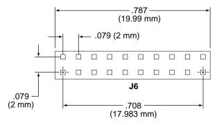
Figure 15. J6 connector dimensions
